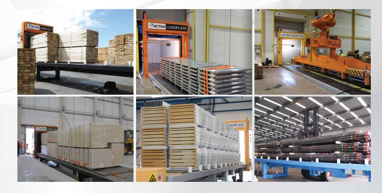
**LoadPlate** is especially suitable for loading complex cargo which is typically difficult to containerize, easily damaged or requires special shipping units such as open top or flat rack containers.
